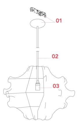
01. RA3690209 – White ceiling rose assembly 02. RF32763 – 3,20 mt of PVC/PVC white cable 3x0,75 03. RF9800200 – Electrical assembly
