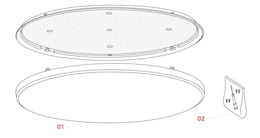
01. RF1570200 – Diffuser 02. RF1570100 – Kit of n. 4 diff. screws & hexagonal screwdriver
