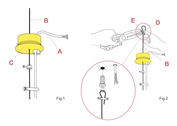
Insert the power supply cable (A) and the steel wire (C) through the ceiling rose (C).
