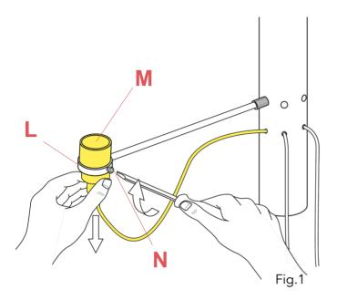
Unfasten the screw (N) and free the lamp holder (M) from the ring of the arm (L) present on the lamp fixture.
