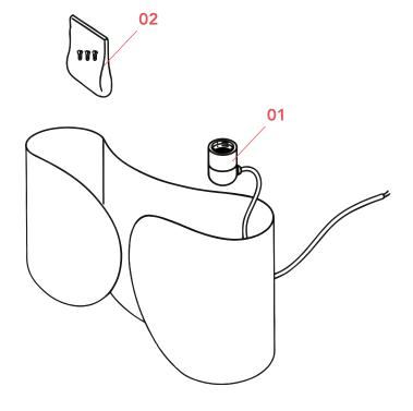
01. RF2400100 - Lamp holder assembly 02. RF06296 - Kit with n.3 screws type M3
