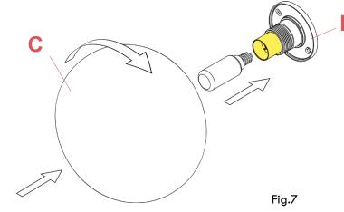
Insert the sheaths (I) in the power supply electrical wires (A). Connect the electrical wires to the lamp holder.
