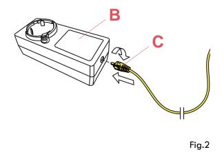
Connect the plug (C) to the power unit (B) locking it in by rotating it  $90^{\circ}$  clockwise.
