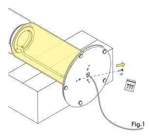
Disconnect the dimmer from the electrical cable.
