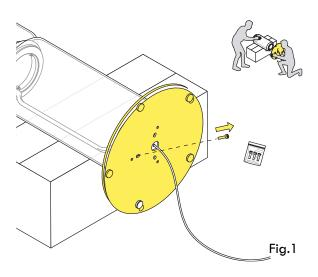
Disconnect the dimmer and the driver from the electrical cable.
