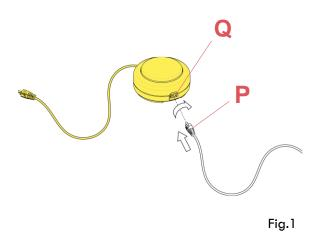
Connect the plug (P) to the push button switch (Q) locking it by turning it  $90^{\circ}$  clockwise.
