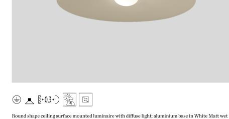
2.1 kg painted; matt texture; steel diffuser; surface Silk Grey wet painted; matt texture; RAL 7044; white opal glass handblown; with COB (Chip on Board) technology for maximum efficiency; phase-cut dim; light colour 3000 K; binning initial MacAdam 2 SDCM; CRI 90; CRI (Colour Rendering Index) 90; degree of protection IP20; PC1; driver included; light source replaceable by an authorized professional; control gear re-
