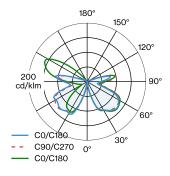
['6342E0GB0'] The technical data represent rated values for an ambient temperature of 25°C. The data values for the luminous flux are initially subject to a tolerance of +/- 10%, those
