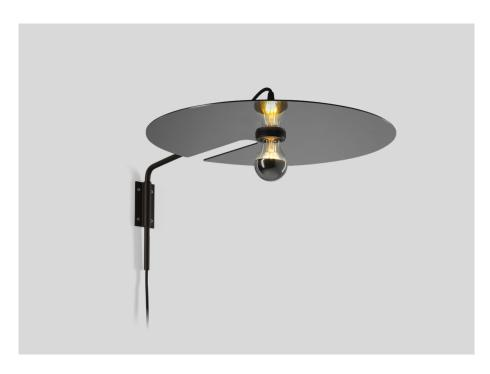
Wall luminaire with extended bracket; surface Black Matt + Black Chrome; powder coated; matt texture; shade: single side reflective aluminium composit panel; black textile cable plug with dimmer; +/-  $35^{\circ}$  tiltable; lamp socket E27; lamp type A60; max. 15W; 220 - 240 V; degree of protection IP20; PC2; lamp not included;
