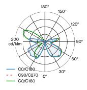
['6342E0NB0'] The technical data represent rated values for an ambient temperature of 25°C. The data values for the luminous flux are initially subject to a tolerance of +/- 10%, those
